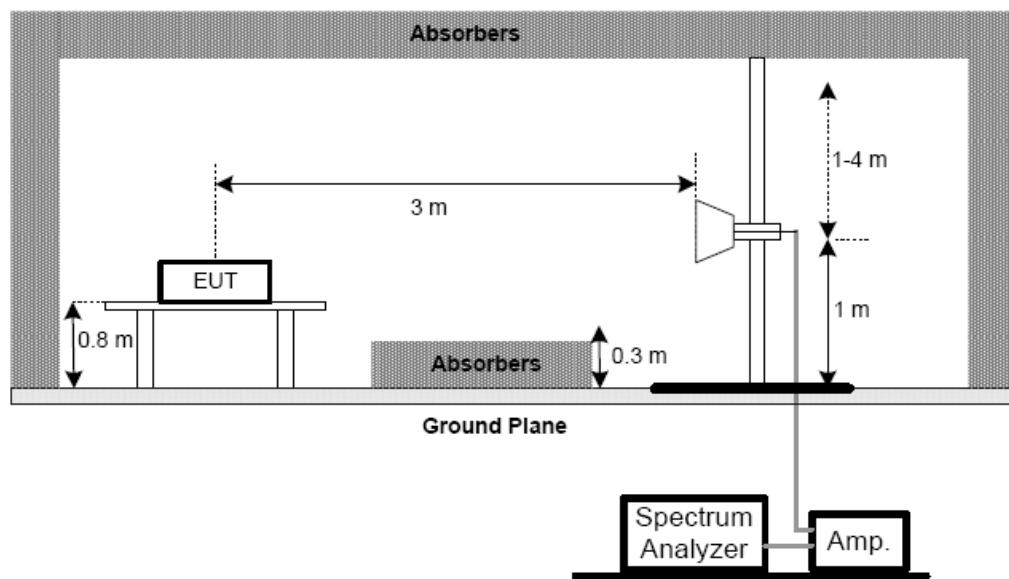
(C) For radiated emissions below 30MHz
