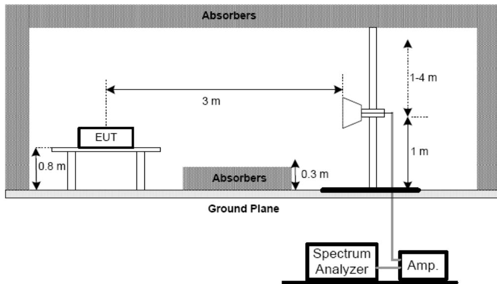
(C) For radiated emissions below 30MHz
