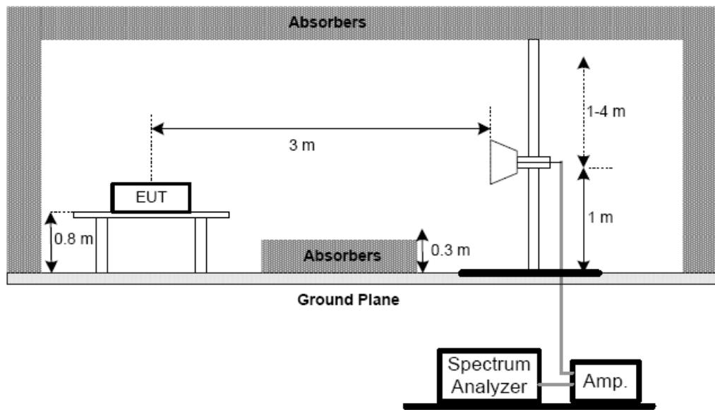
(C) For radiated emissions below 30MHz
