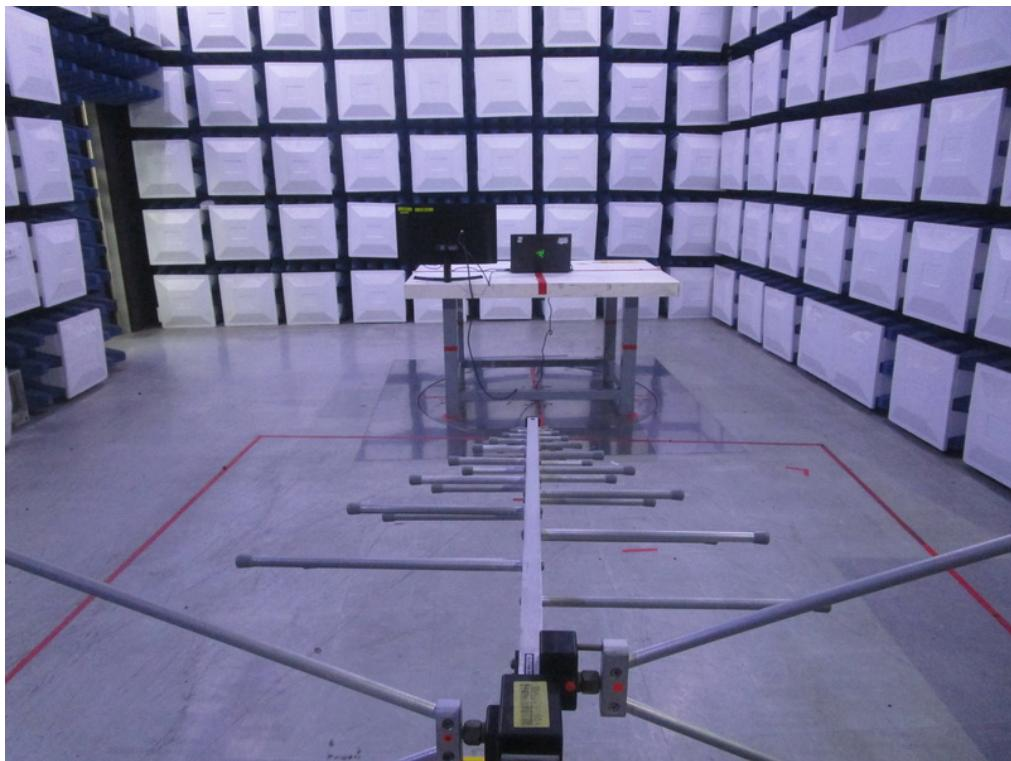
**Radiated Emissions Test Photos****Above 1 GHz**
