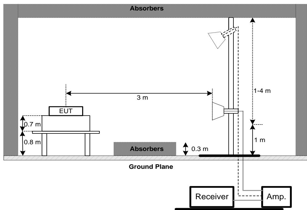
(C) For radiated emissions below 30MHz
