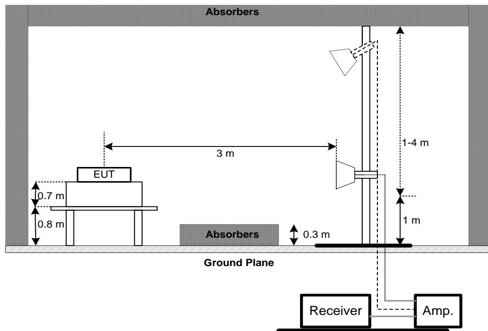
(C) For Radiated Emissions Below 30MHz
