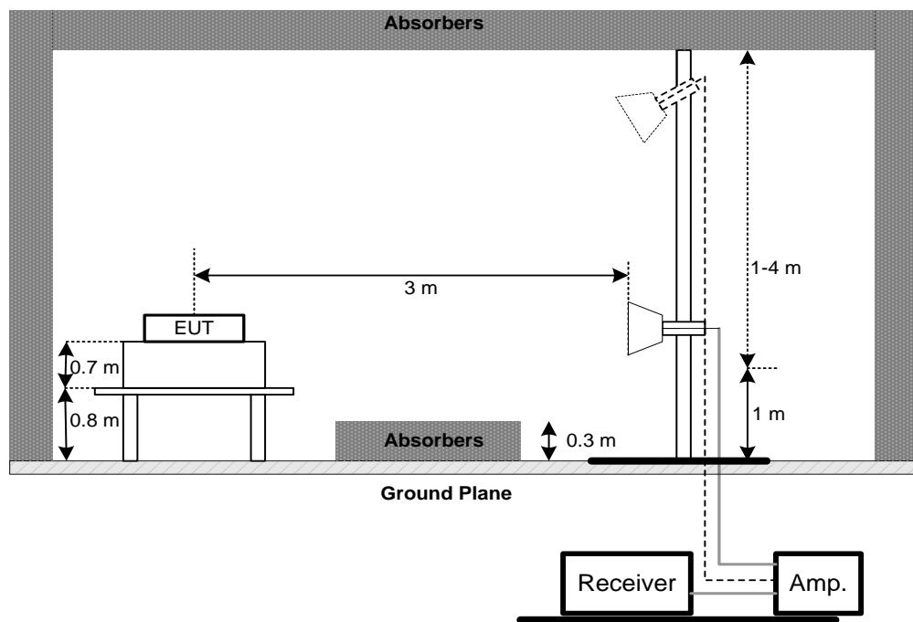
(C) For Radiated Emissions Below 30MHz
