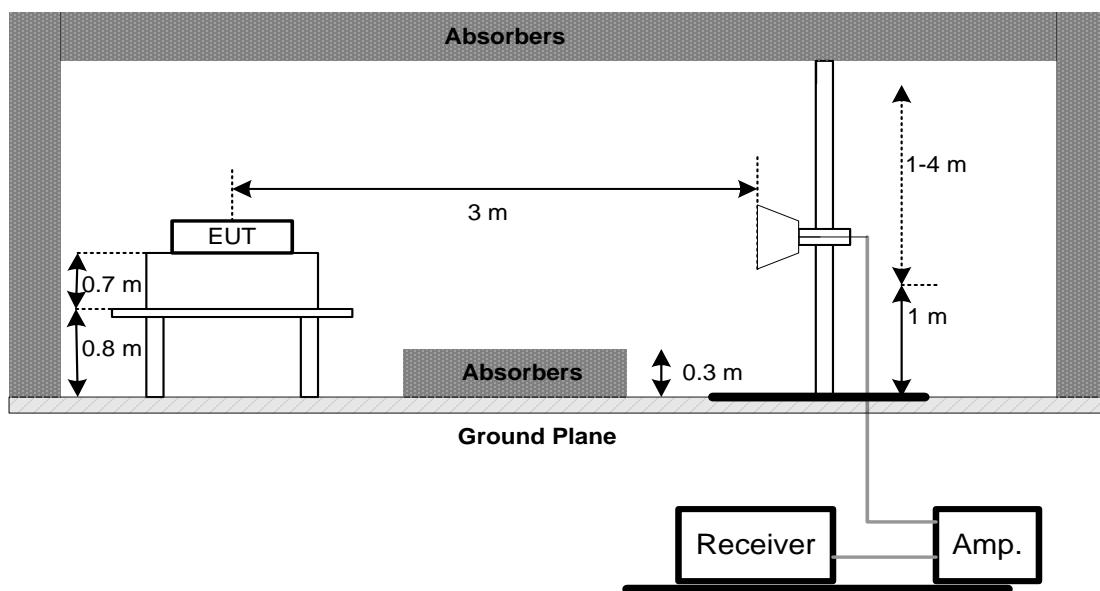
(C) For radiated emissions below 30MHz
