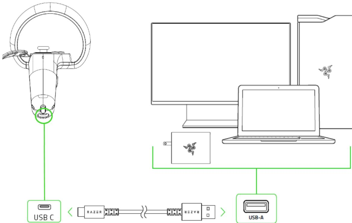
**i** For best results, use the charging cable that comes with the VR Controller to connect it to a source that can supply 6 watts (5 volts, 1.2 amps) of power.
