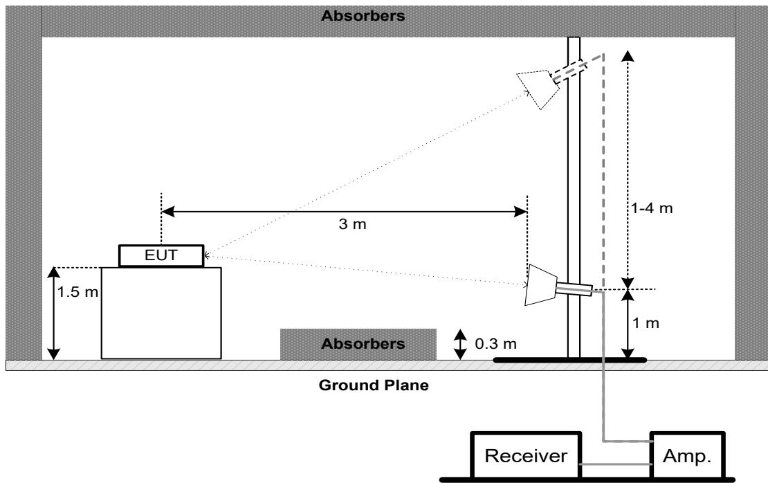
**Harmonic(18 GHz to 26.5 GHz)**
