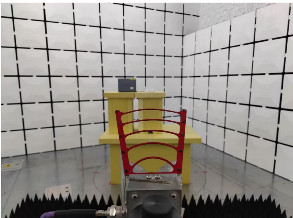
**Radiated Emissions Test Photos****Above 1 GHz\_ Harmonic (18 GHz to 26.5 GHz)**
