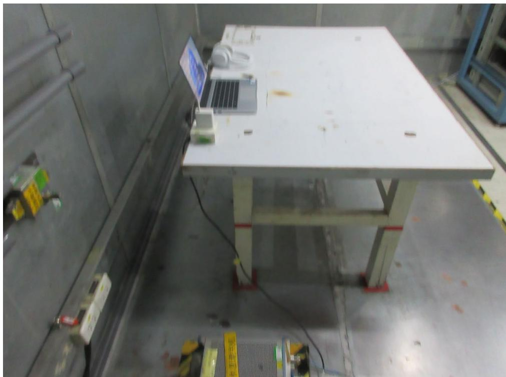
**Radiated Emissions Test Photos****30 MHz to 1000 MHz**
