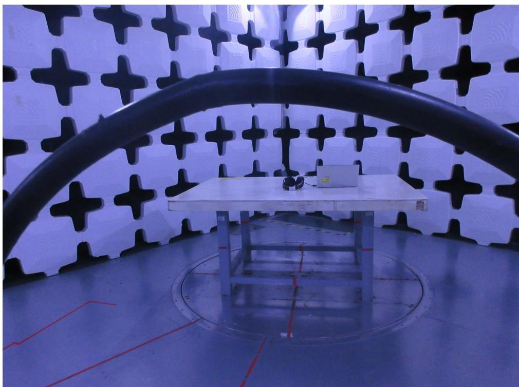
**Radiated Emissions Test Photos****30 MHz to 1000 MHz**
