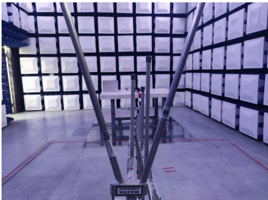
**Radiated Emissions Test Photos****Above 1 GHz**
