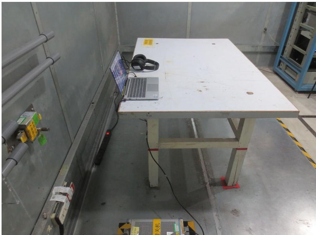
**Radiated Emissions Test Photos****9 kHz to 30 MHz**
