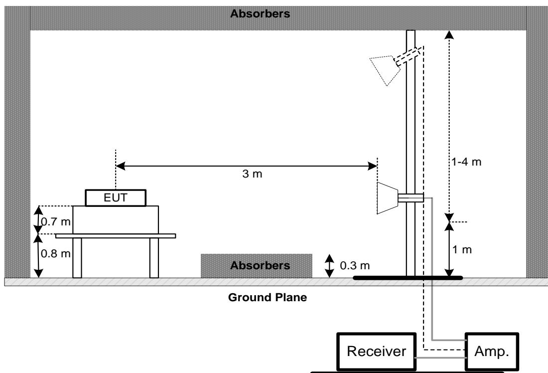
(C) For Radiated Emissions Below 30MHz
