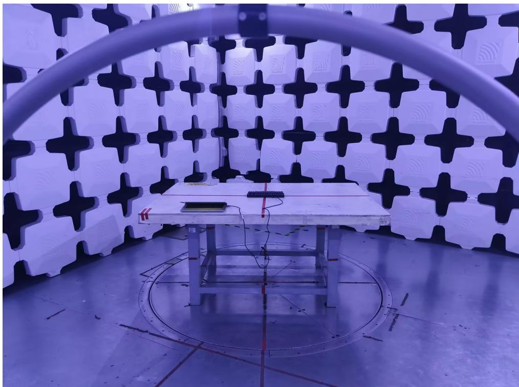
**Radiated Emissions Test Photos****30 MHz to 1000 MHz**
