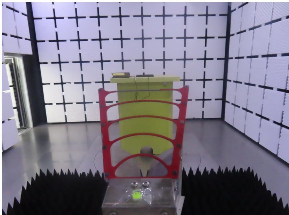
**Radiated Emissions Test Photos****Harmonic(18 GHz to 26.5 GHz)**
