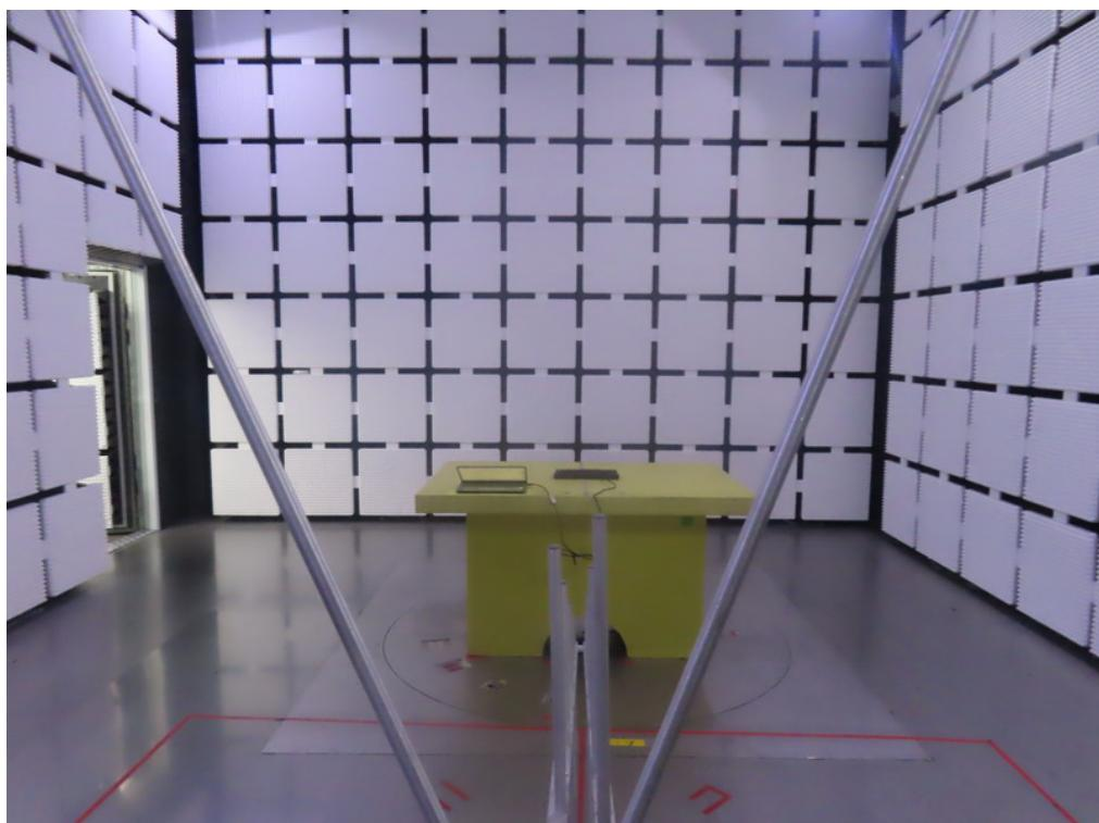
**Radiated Emissions Test Photos****Band edge & Harmonic(1 GHz to 18 GHz)**
