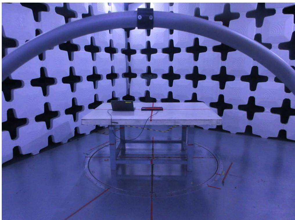
**Radiated Emissions Test Photos****30 MHz to 1000 MHz**
