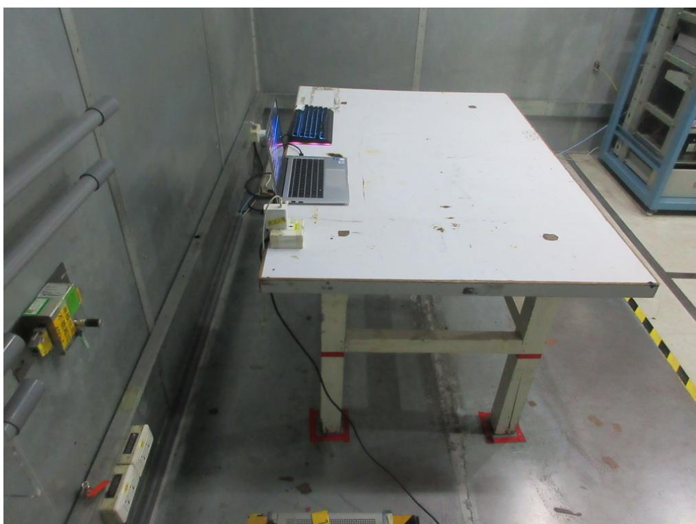
**Radiated Emissions Test Photos****9 kHz to 30 MHz**
