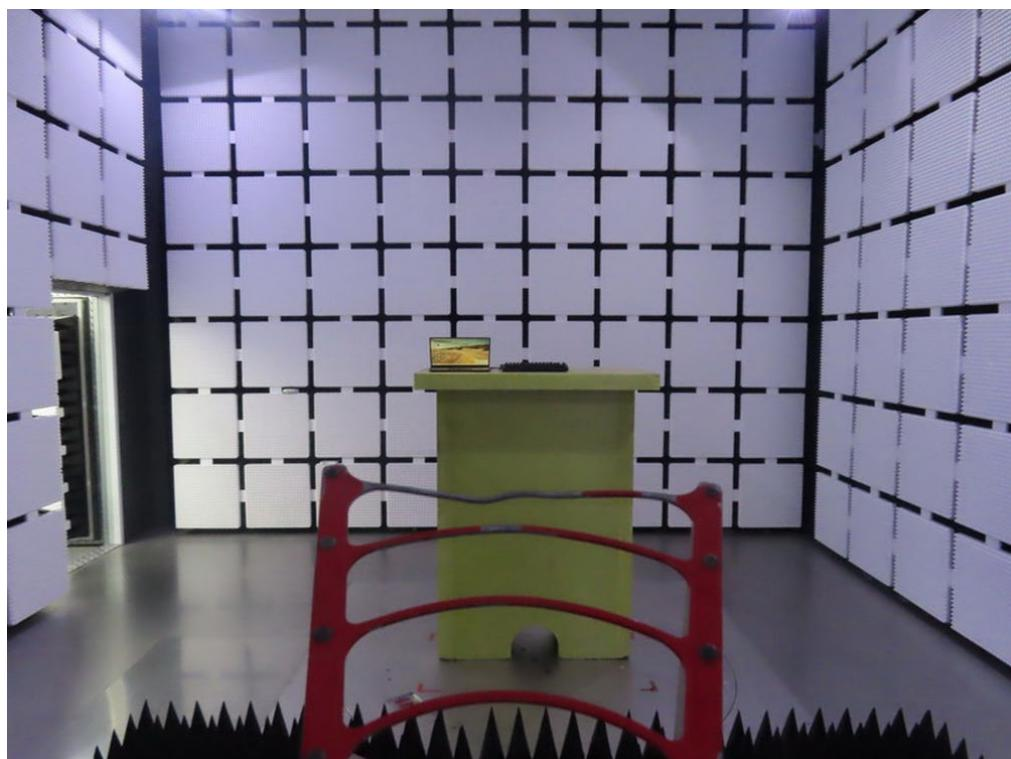
**Radiated Emissions Test Photos****Above 18 GHz****(Harmonic)**
