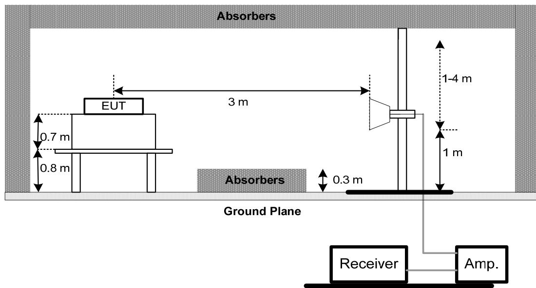
(C) For radiated emissions below 30MHz
