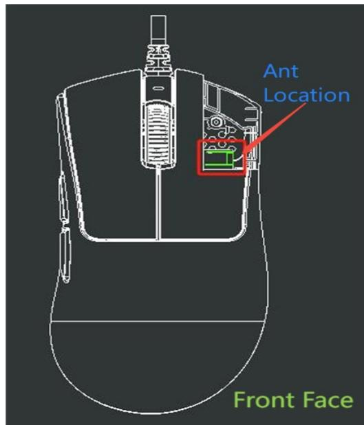
Note: The EUT only has one antenna and does not have synchronous transmission function.
