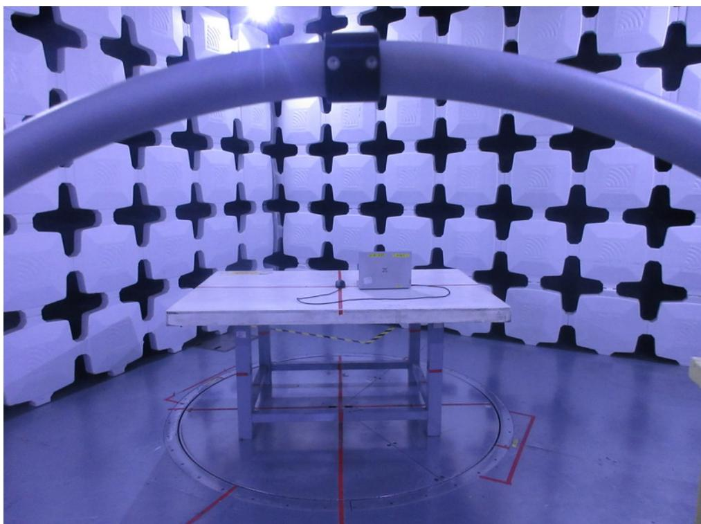
**Radiated Emissions Test Photos****30 MHz to 1000 MHz**
