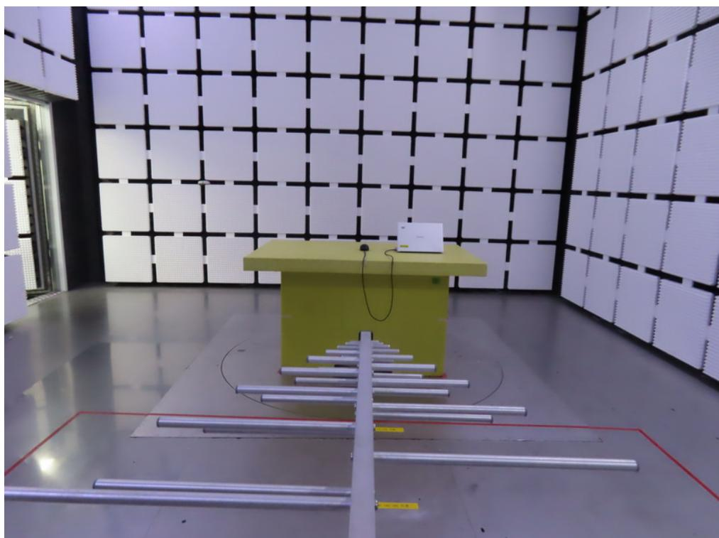
**Radiated Emissions Test Photos****Above 1 GHz**
