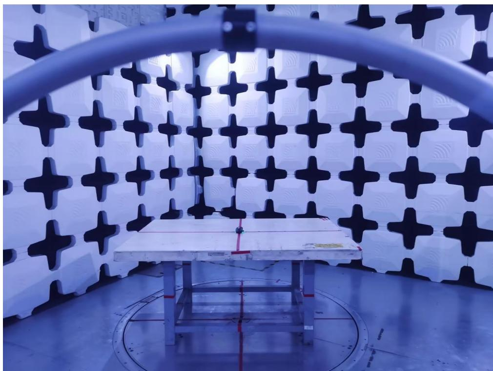
**Radiated Emissions Test Photos****30 MHz to 1000 MHz**
