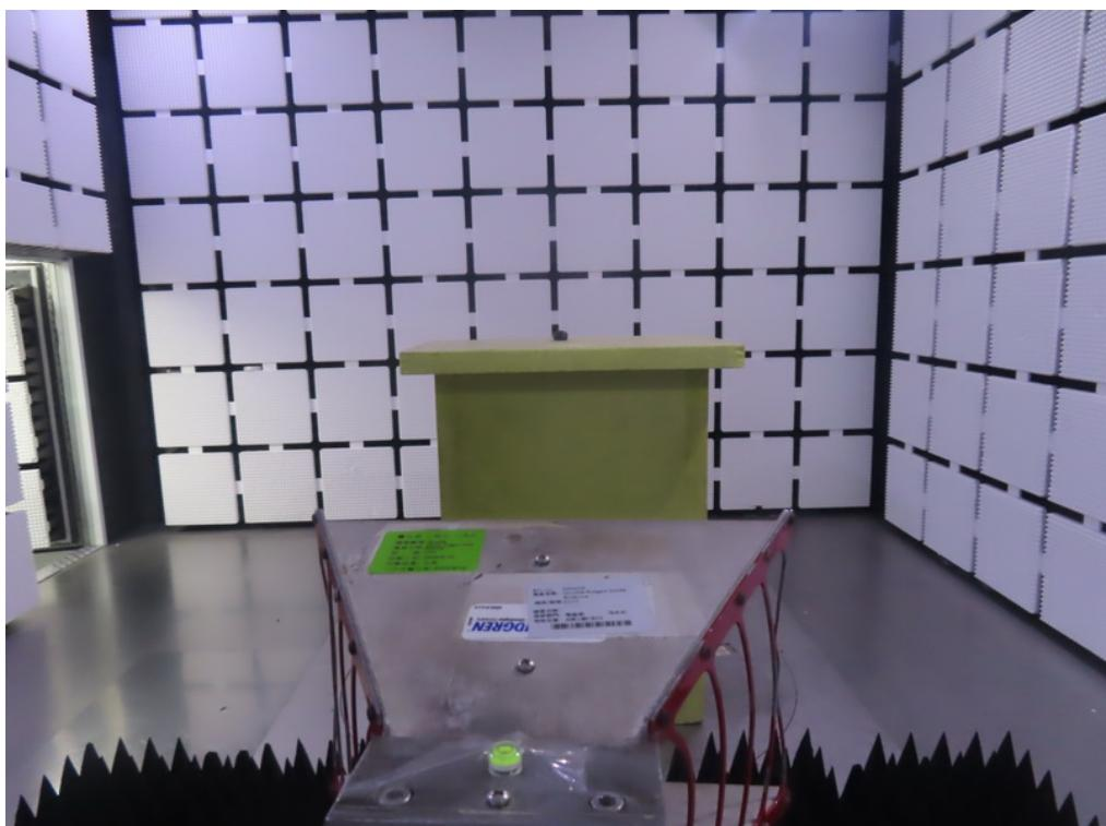
**Radiated Emissions Test Photos****Above 1 GHz\_ Harmonic (18 GHz to 26.5 GHz)**
