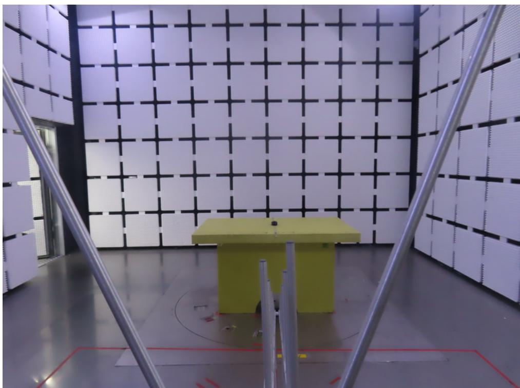
**Radiated Emissions Test Photos****Above 1 GHz\_ Band edge & Harmonic (1 GHz to 18 GHz)**
