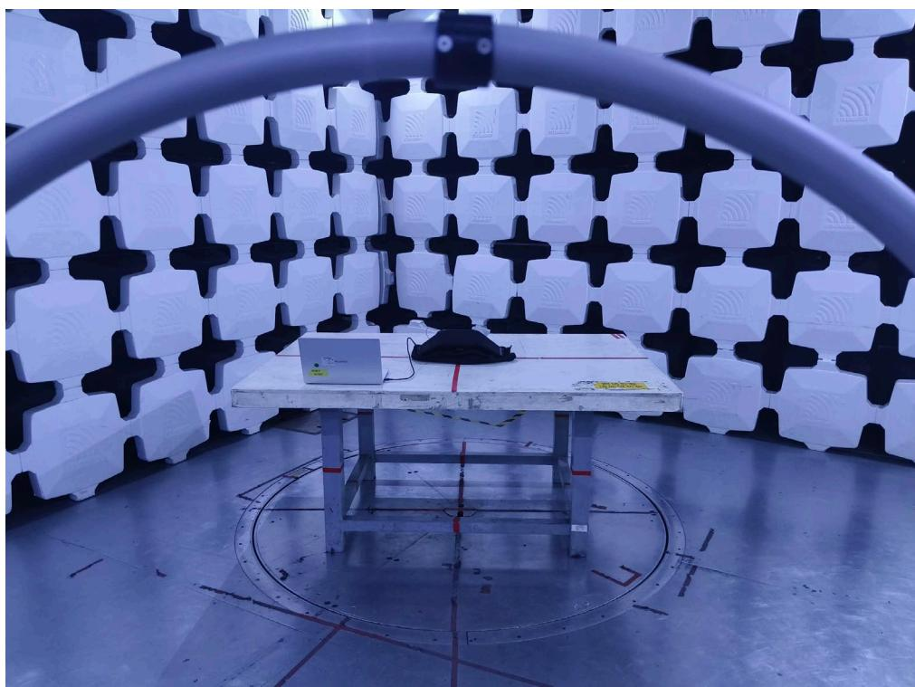
**Radiated Emissions Test Photos****30 MHz to 1000 MHz**
