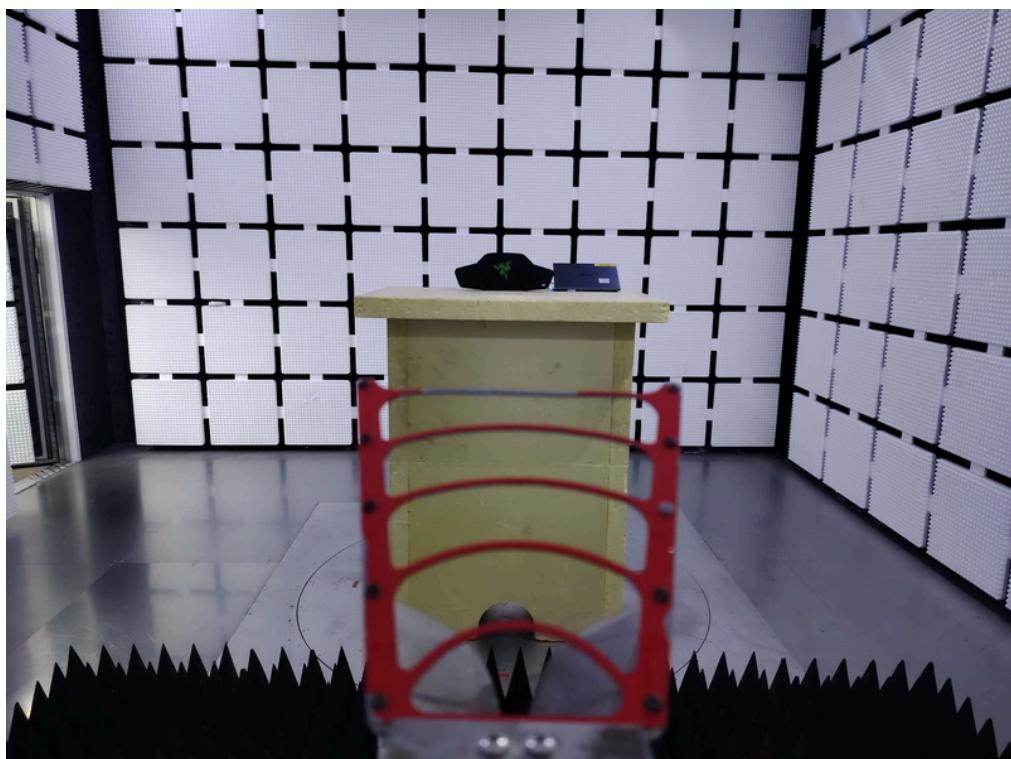
**Radiated Emissions Test Photos****Above 18 GHz****(Harmonic)**
