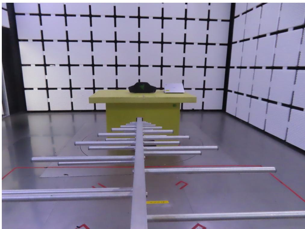
**Radiated Emissions Test Photos****1 GHz -18 GHz****(Band edge & Harmonic)**
