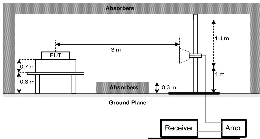
(C) For radiated emissions below 30MHz
