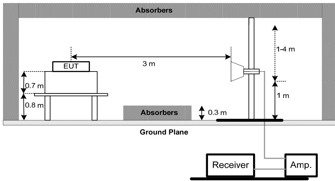
(C) For radiated emissions below 30MHz
