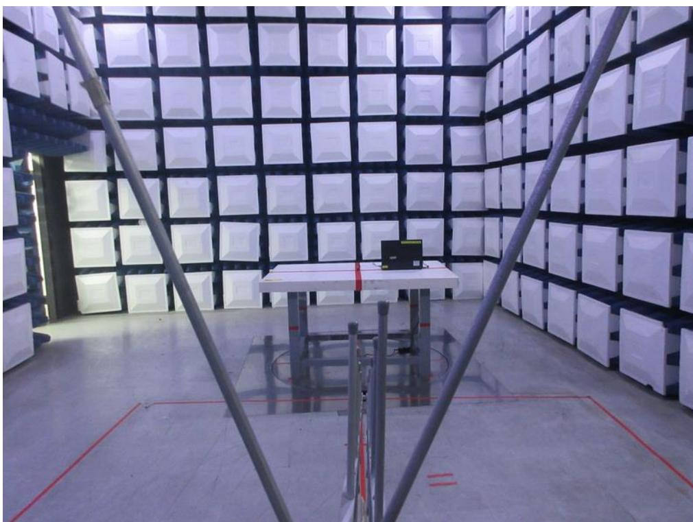
**Radiated Emissions Test Photos****Above 1 GHz**
