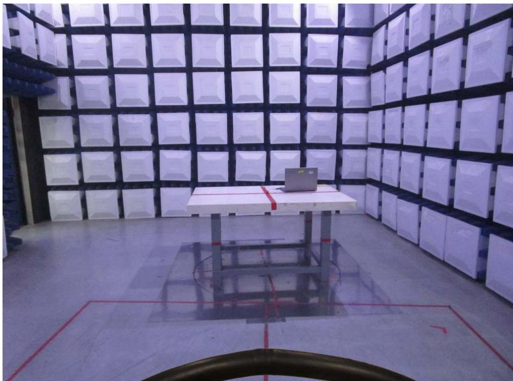
**Radiated Emissions Test Photos****30 MHz to 1000 MHz**
