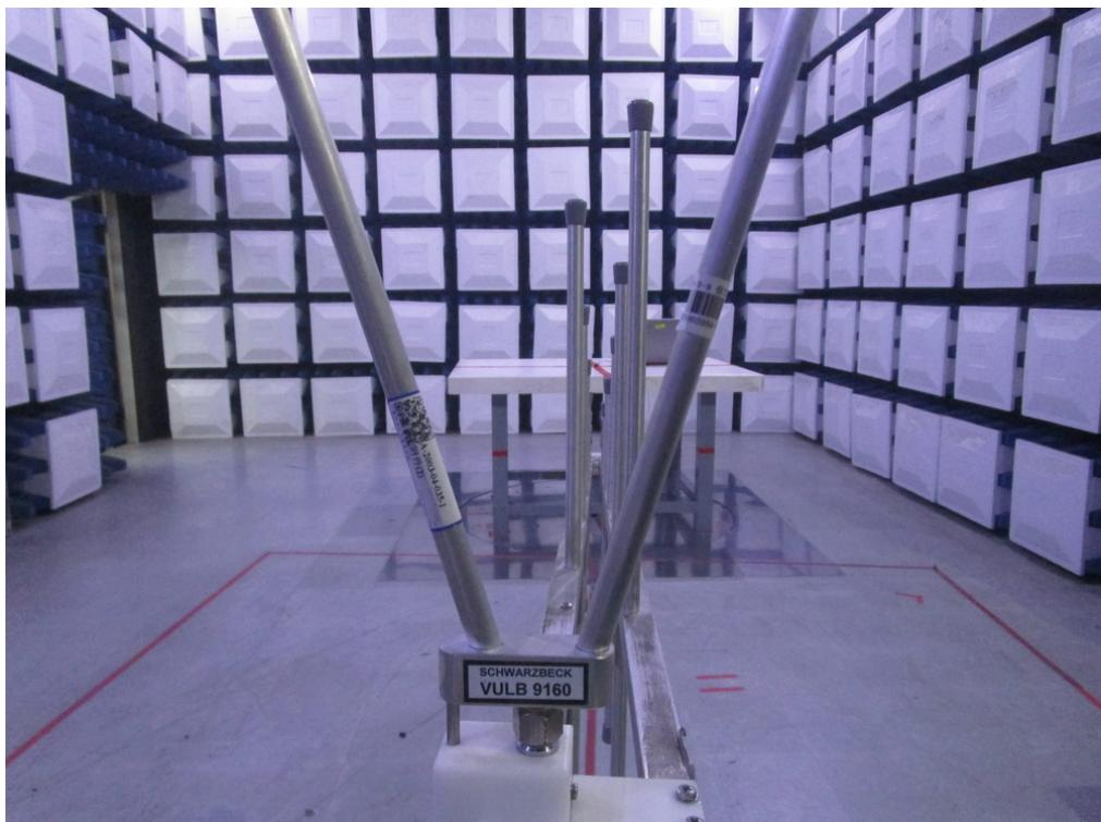
**Radiated Emissions Test Photos****Above 1GHz**
