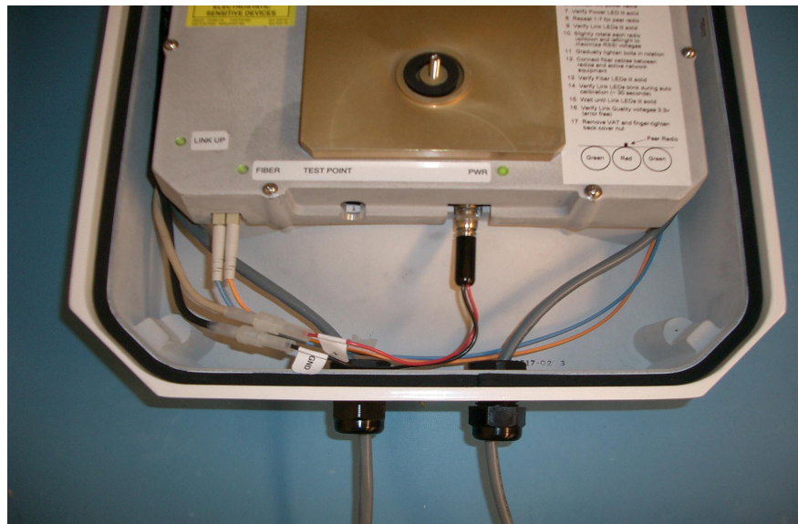
Figure 3-8: Inside view of fiber and power cable connected E60 or E60X unit
