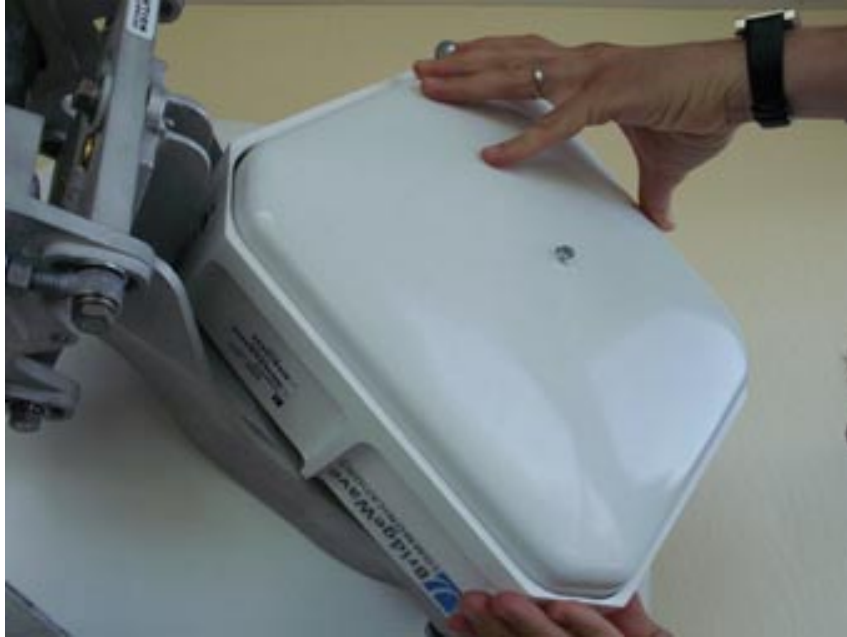
Figure 3-10.1 Attaching the radio to the back of the antenna
