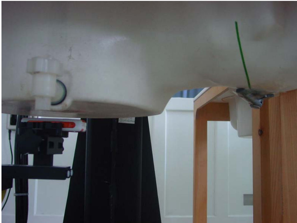
Picture B3: Body-worn Position with Bluetooth transmitter (towards ground, the distance from handset to the bottom of the Phantom is 1.5cm)
