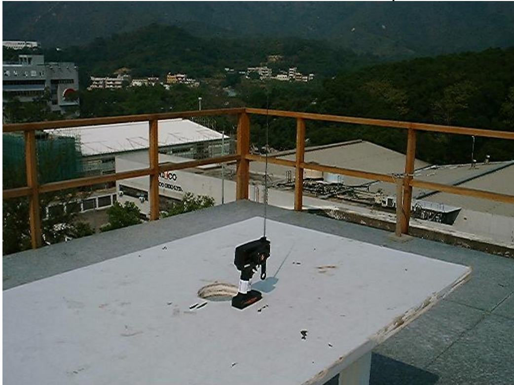
Measurement of Radiated Emission Test Set Up
