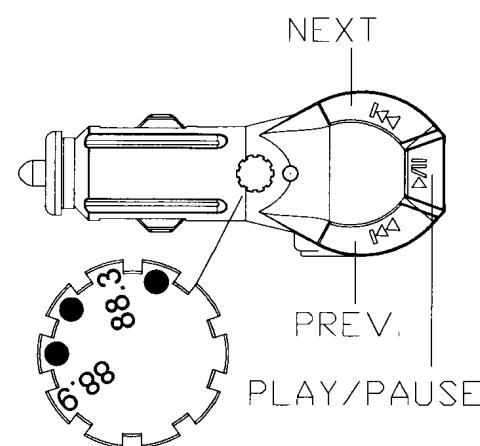
Channel rotary switch setting list
