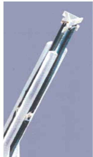
Inside view of ES3DV2 E-field Probe
