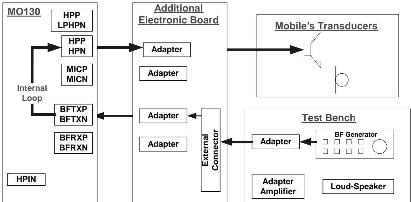
If the final product uses a second speaker for incoming call ringing, the functional test could be as following schematic :
