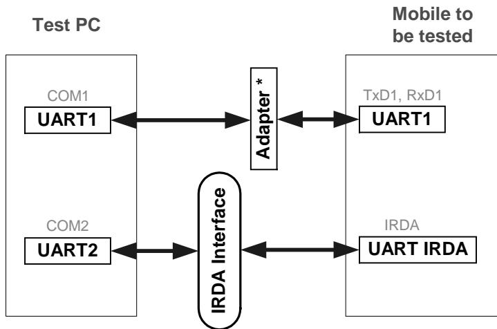
\* : used to shift and adjust the level of the signals
