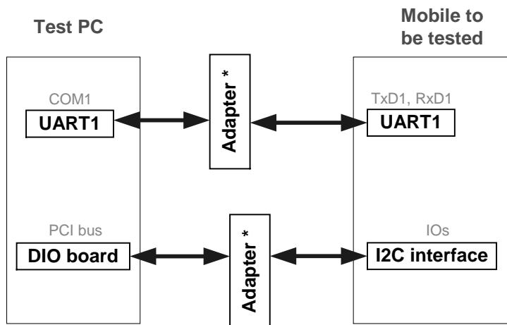
\* : used to shift and adjust the level of the signal s
