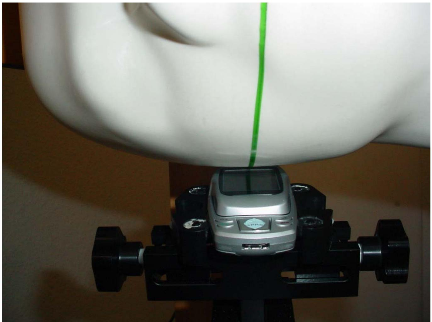
Annex 3.2 Test mode 2 : head measurement, EUT opened
