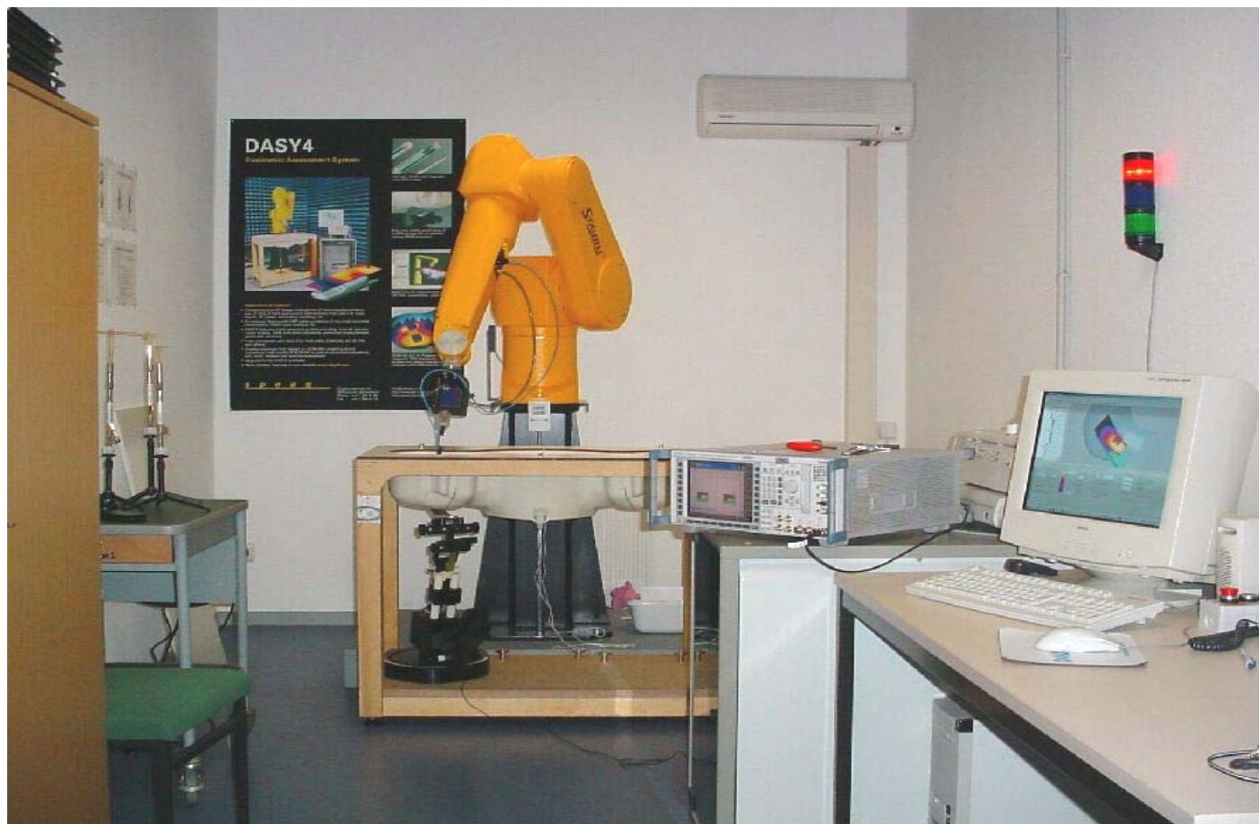
Annex 3.1 Test mode 1 : head measurement, EUT closed
