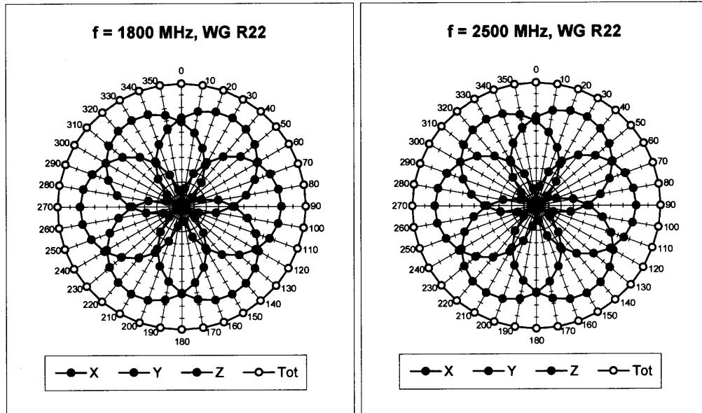
**Isotropy Error ( $\phi$ ),  $\theta = 0^\circ$**
