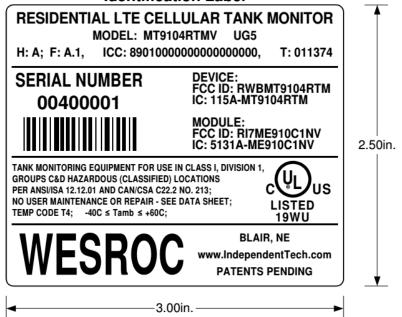
Label printed on Brady B489 polyester label stock using Brady 4300 Series thermal transfer ribbon.
