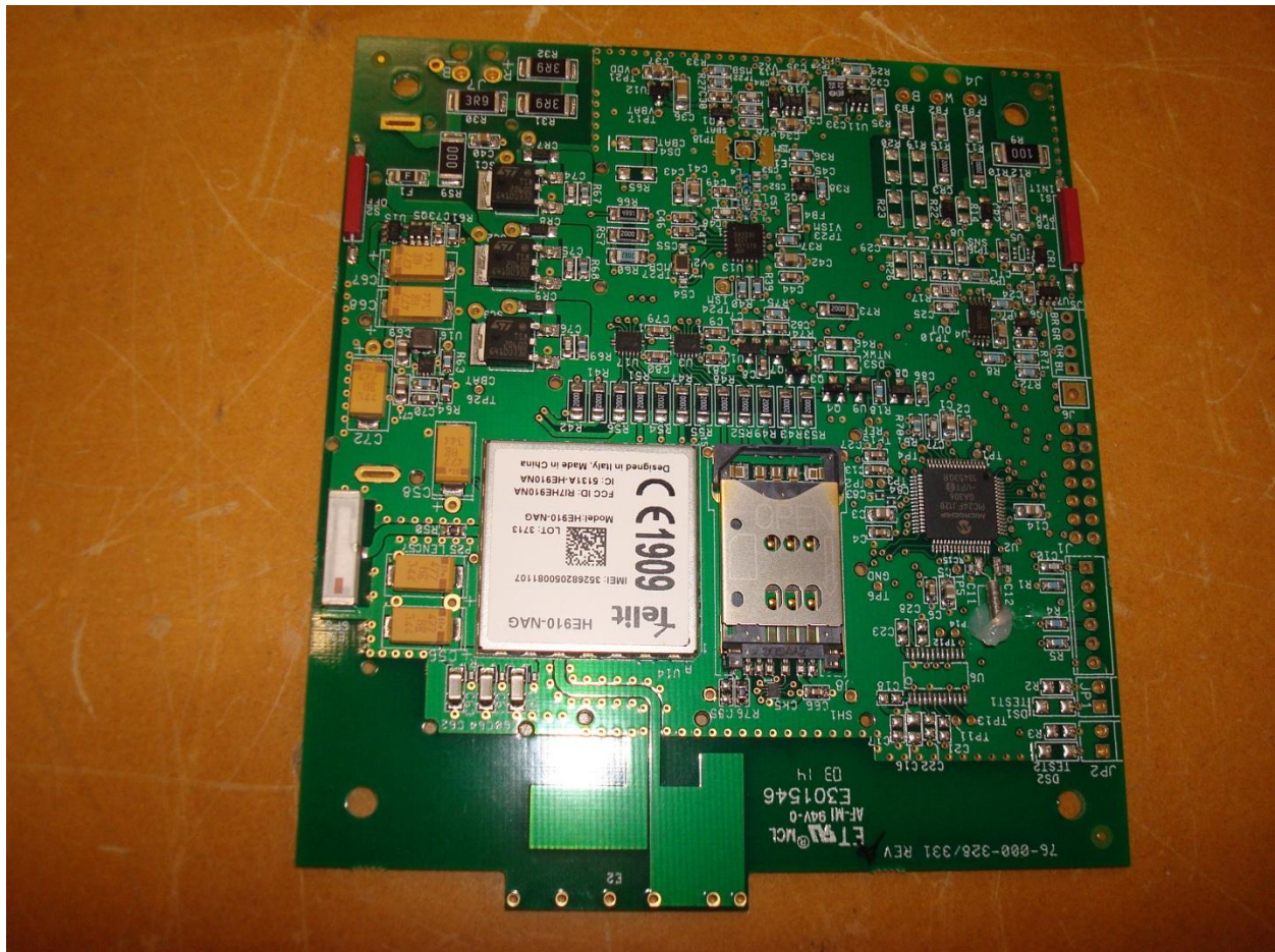
Figure 11 - Circuit board - unpotted, antenna removed
