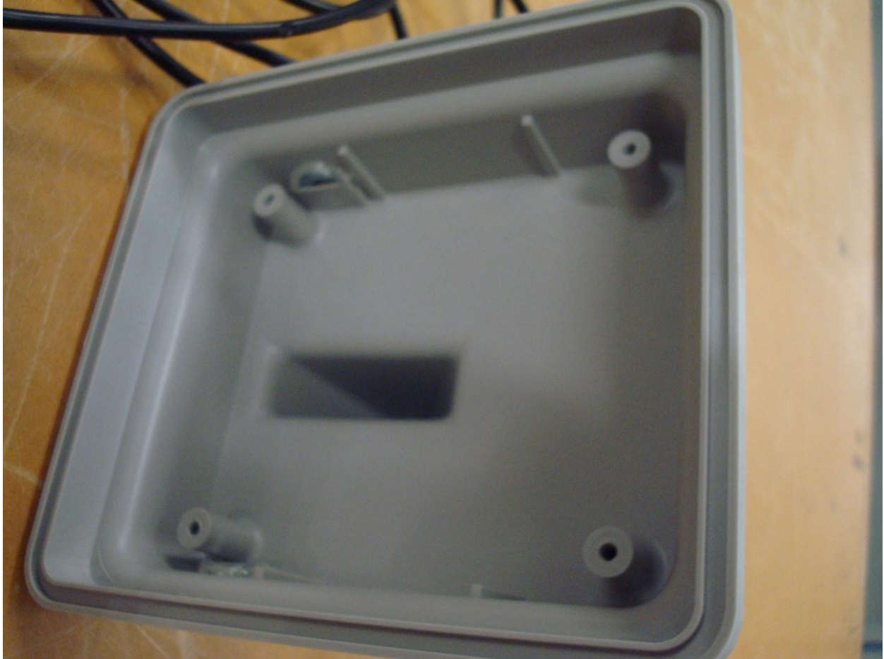
Figure 3 - Inside of the top part of the plastic enclosure
