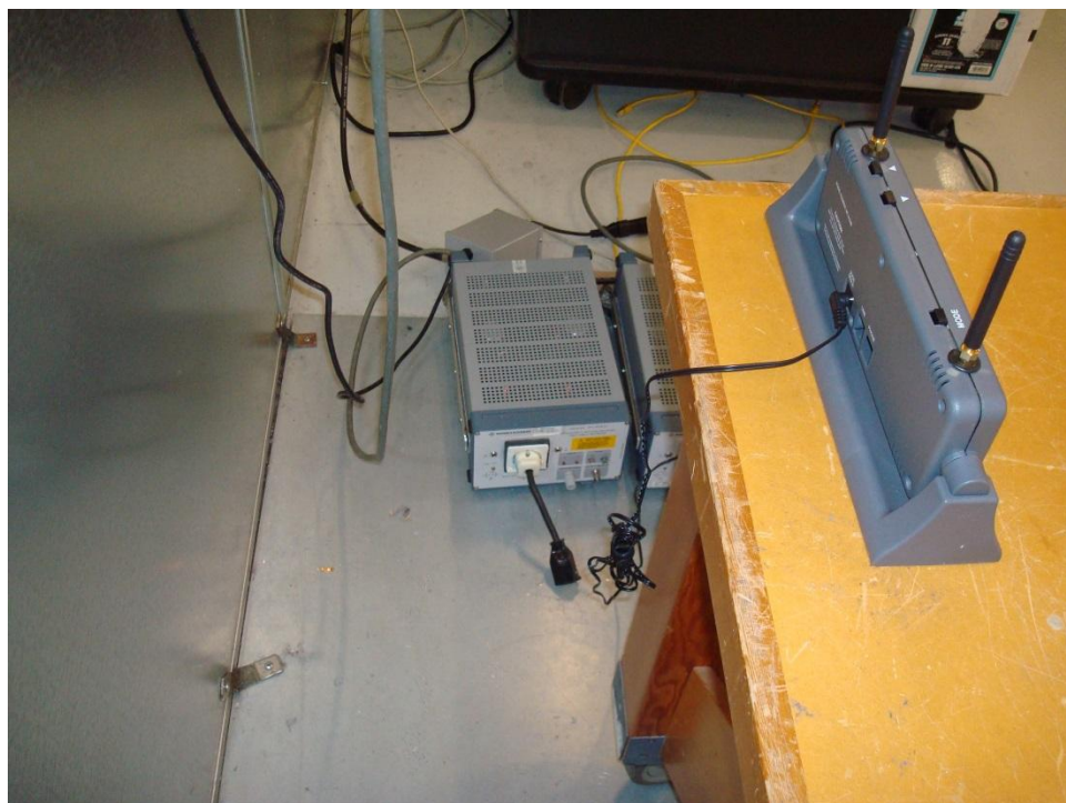
Figure 23 - Conducted Emissions Test Setup
