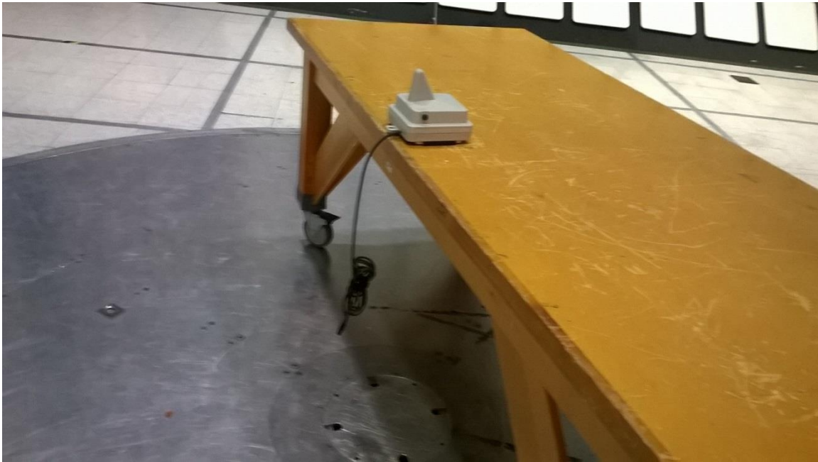
Figure 13 - Radiated Emissions Test Setup, 30MHz to 1GHz Table height was 0.8m
