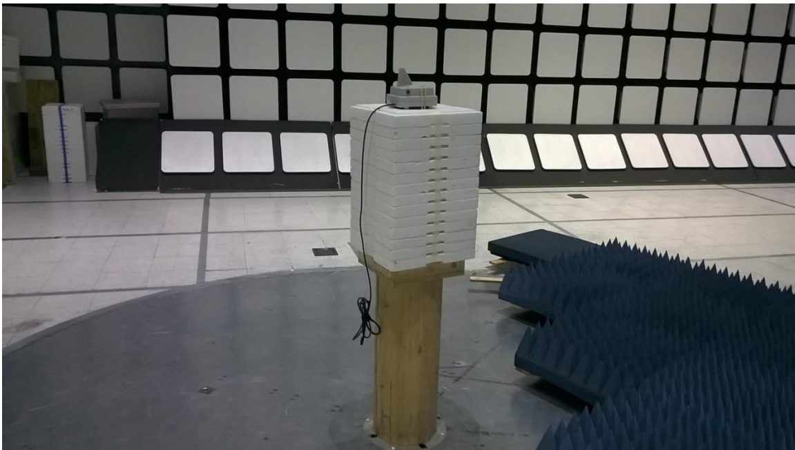
Figure 14 - Radiated Emissions Test Setup, 1 – 10GHz Table height was 1.5m
