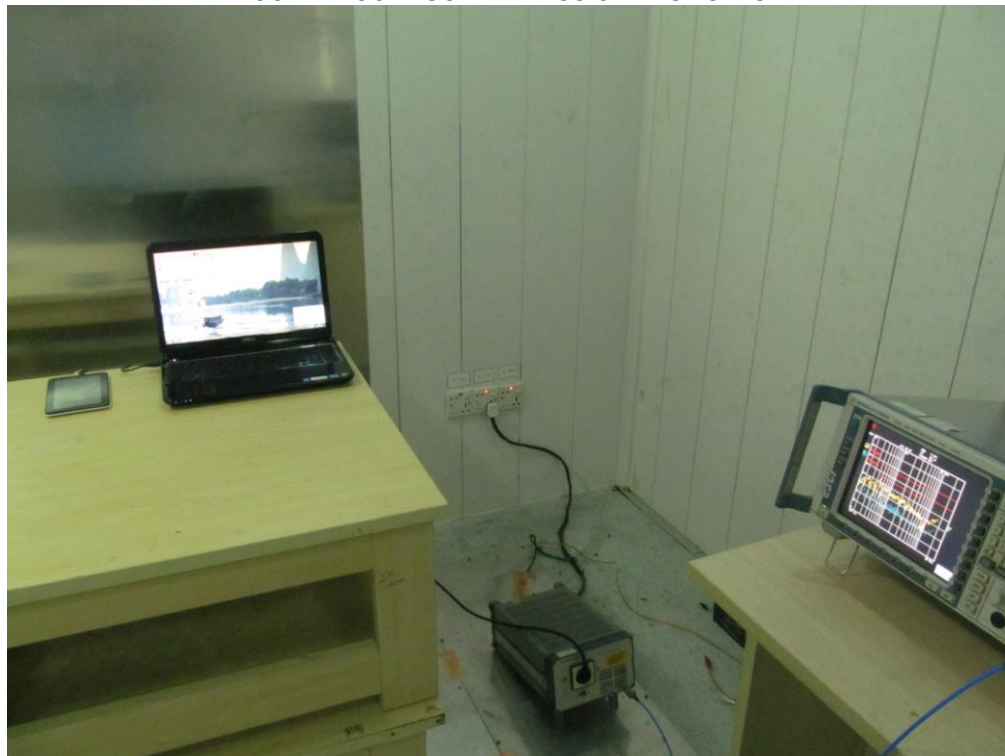
FCC RADIATED EMISSION TEST SETUP
