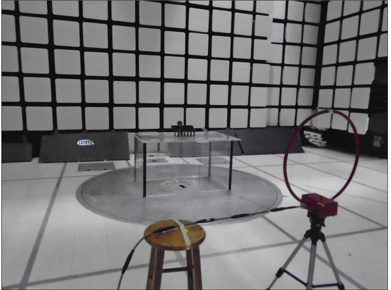
Photograph 1. Radiated Spurious Emissions Setup, 9 kHz – 30 MHz
