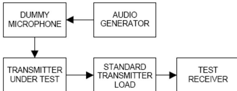
Input 2500Hz signal to the microphone, adjust level to 50% rated deviation , add the level 16dB, test this status the 99% occupied bandwidth and record it.
