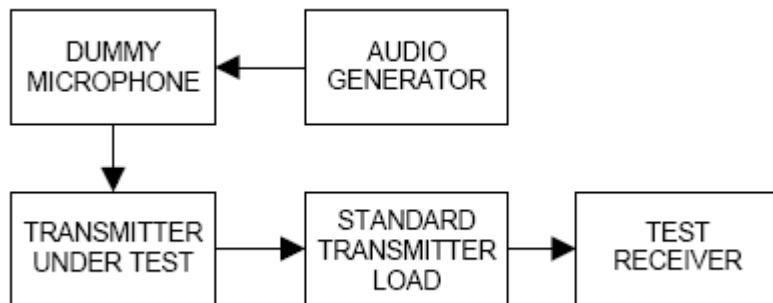
Test at 9 different modulating frequencies (100Hz, 300Hz, 500Hz, 1kHz, 2.5kHz, 5kHz, 10kHz, 15kHz, 20kHz), the output level of the audio generator was varied up to 600 mV and the FM deviation level was recorded as below.
