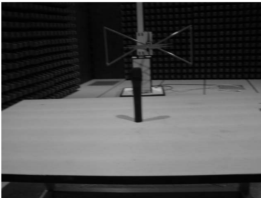
Photograph 1: Set-up for Radiation Measurement Below 1GHz
