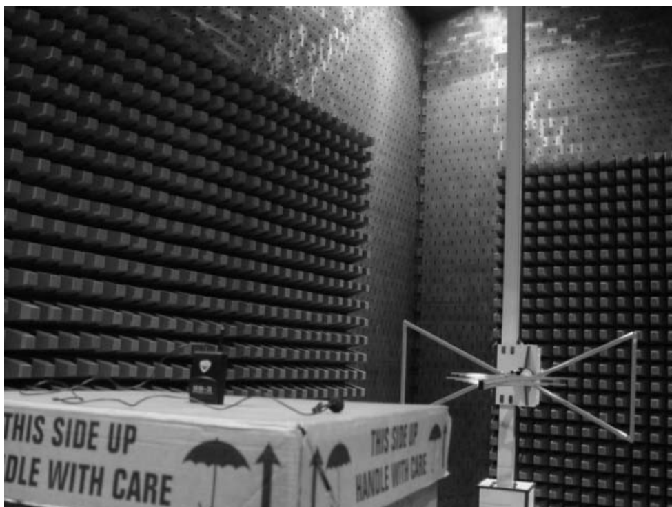
Photograph 1: Set-up for Radiation Measurement Below 1GHz
