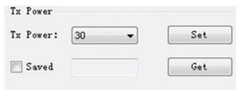
Picture 7 RF output power setting
