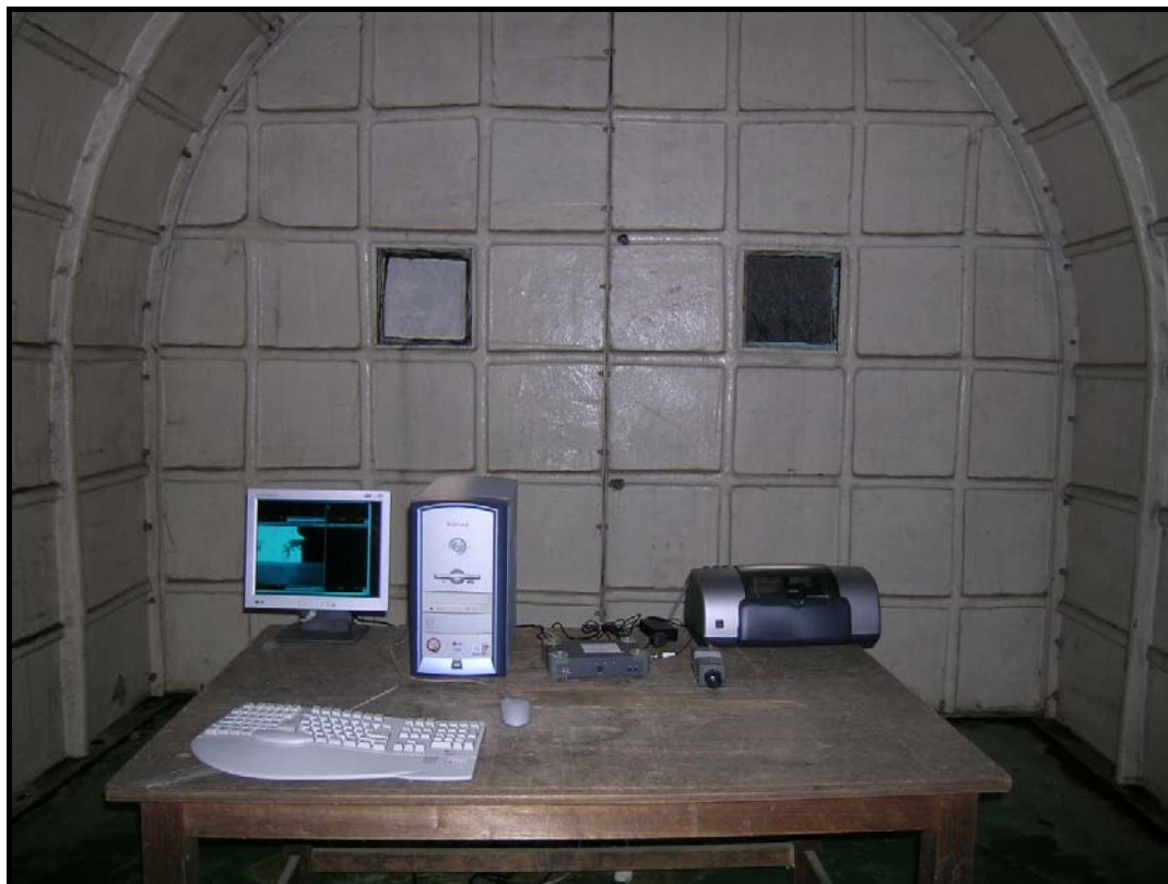
Photograph 2: Setup for Radiated Emissions
