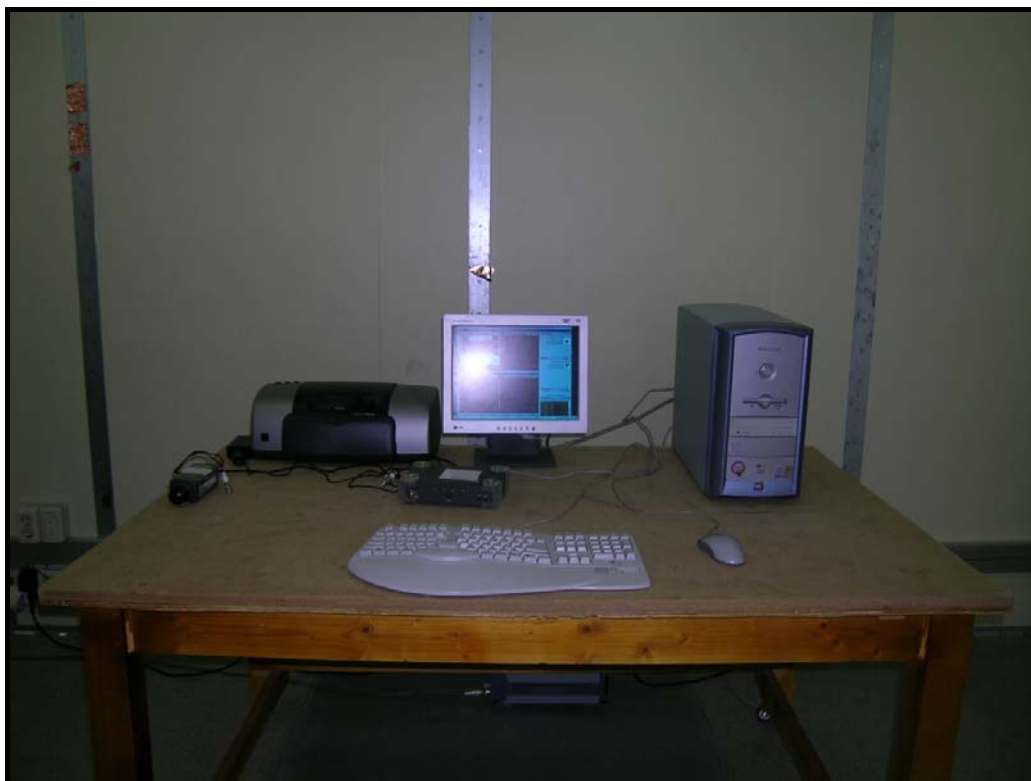
Photograph 1: Setup for Conducted Emissions
