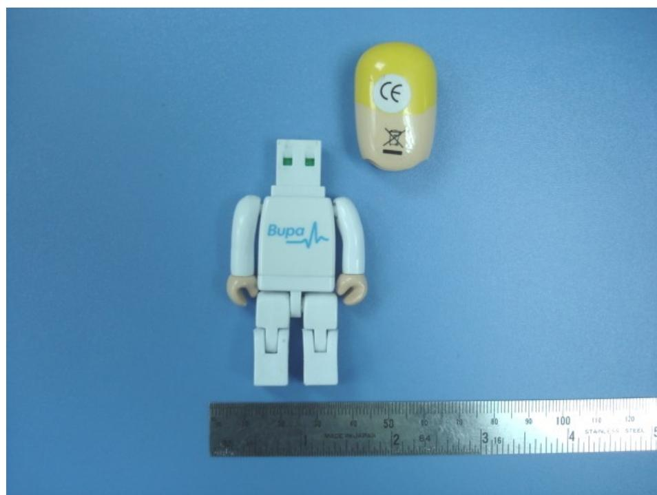
Because the majority of the device housing is too small, there is extremely limited space available to attach the required label carrying both the FCC identifier and statement. For this reason **Sweda Limited** proposes placing FCC statement in the user manual.
