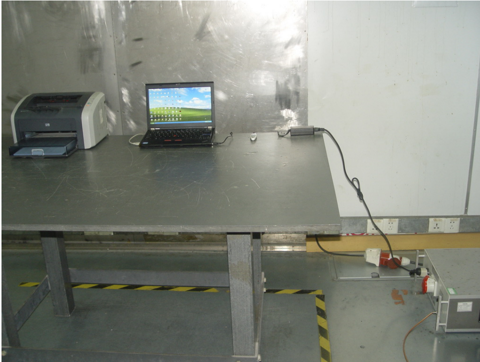
Photograph 6: Set-up for Radiated Emissions, below 1GHz
