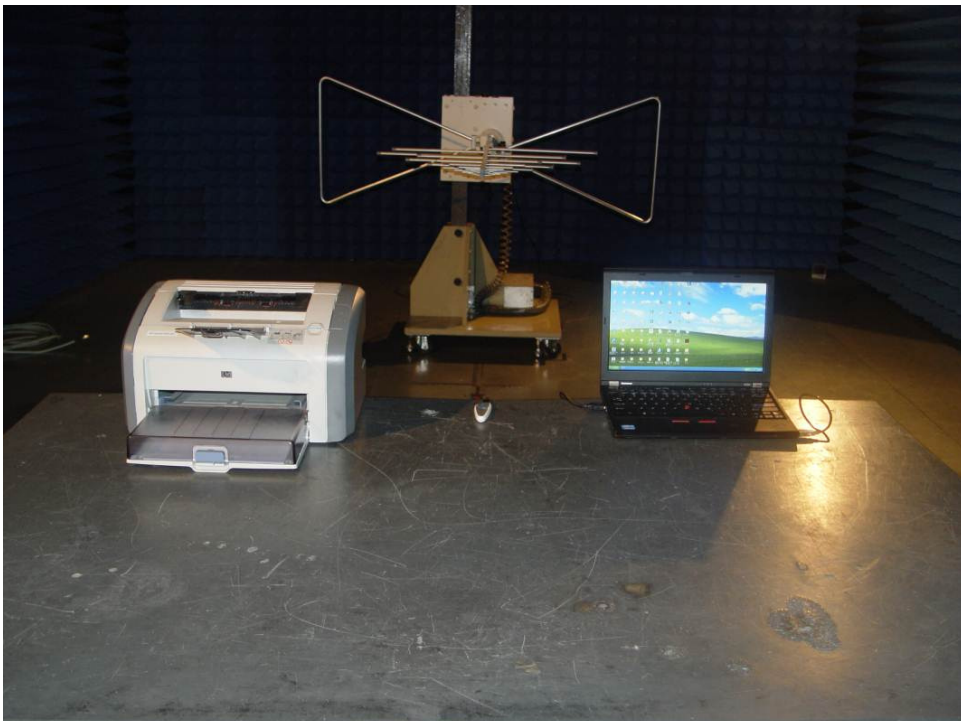
Photograph 6: Set-up for Radiated Emissions, below 1GHz
