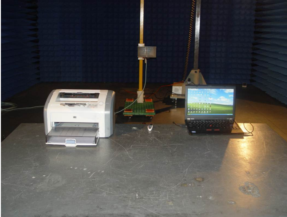
Photograph 7: Set-up for Radiated Emissions, above 1GHz
