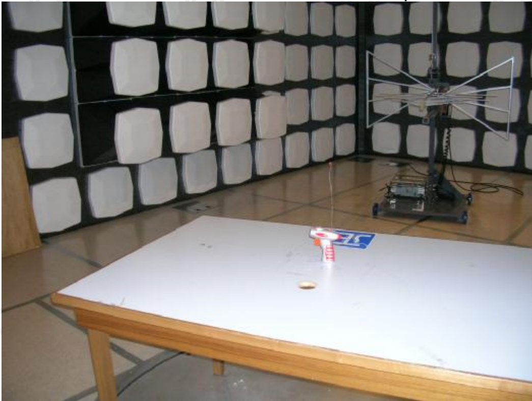
Measurement of Radiated Emission Test Set Up
