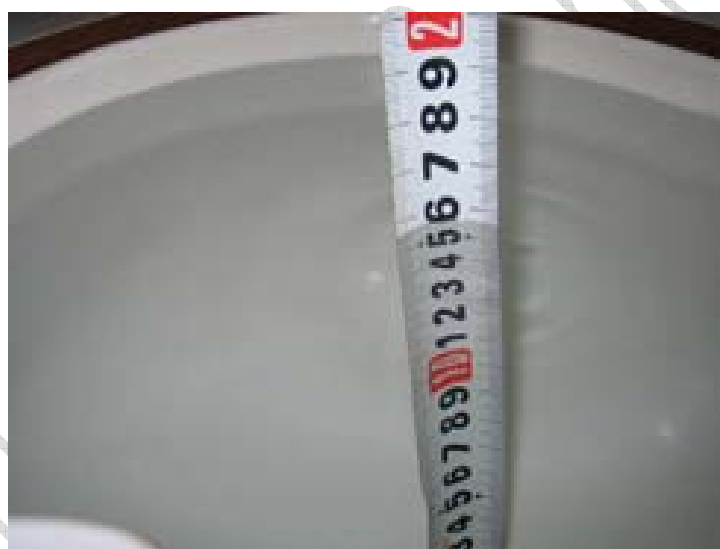
Picture 17 Liquid Depth at Ear Reference Point for 1900MHz Head Liquid
