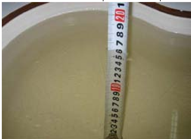
Picture 16 Liquid Depth at Ear Reference Point for 835MHz Head Liquid
