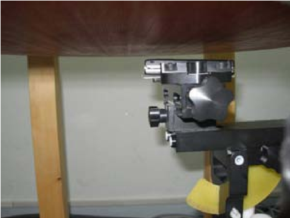
Picture 7 Body-Worn mode with Back towards Phantom 1.5cm
