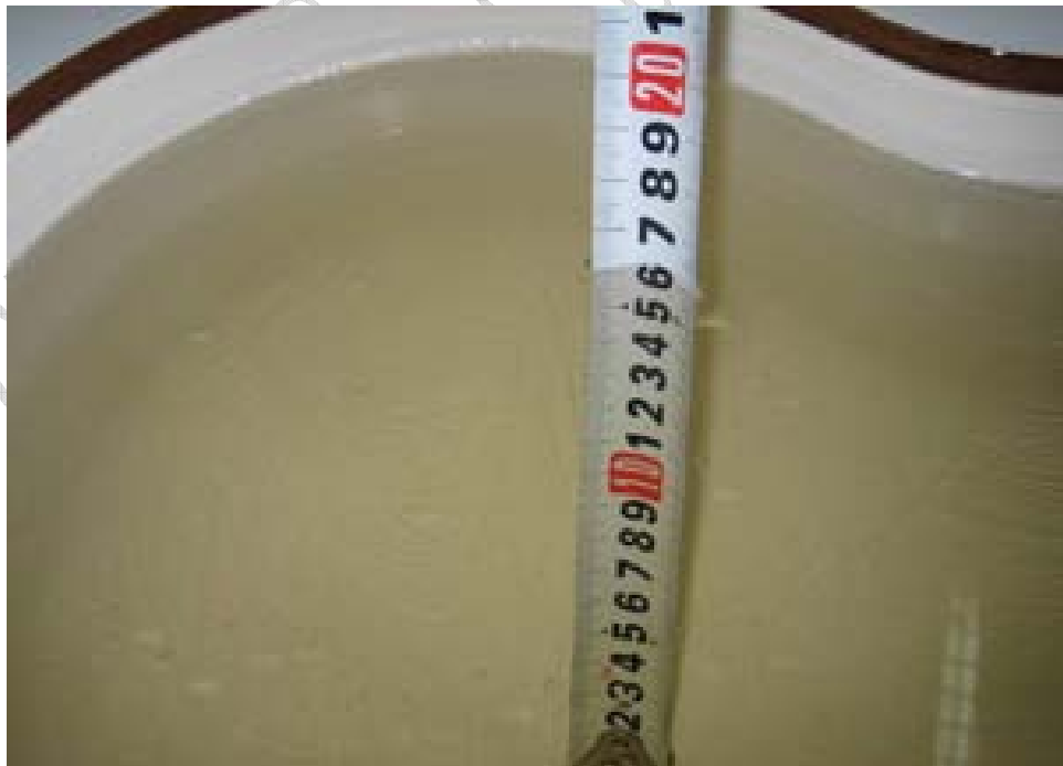
Picture 8 Liquid Depth at Ear Reference Point for 835MHz Head Liquid
