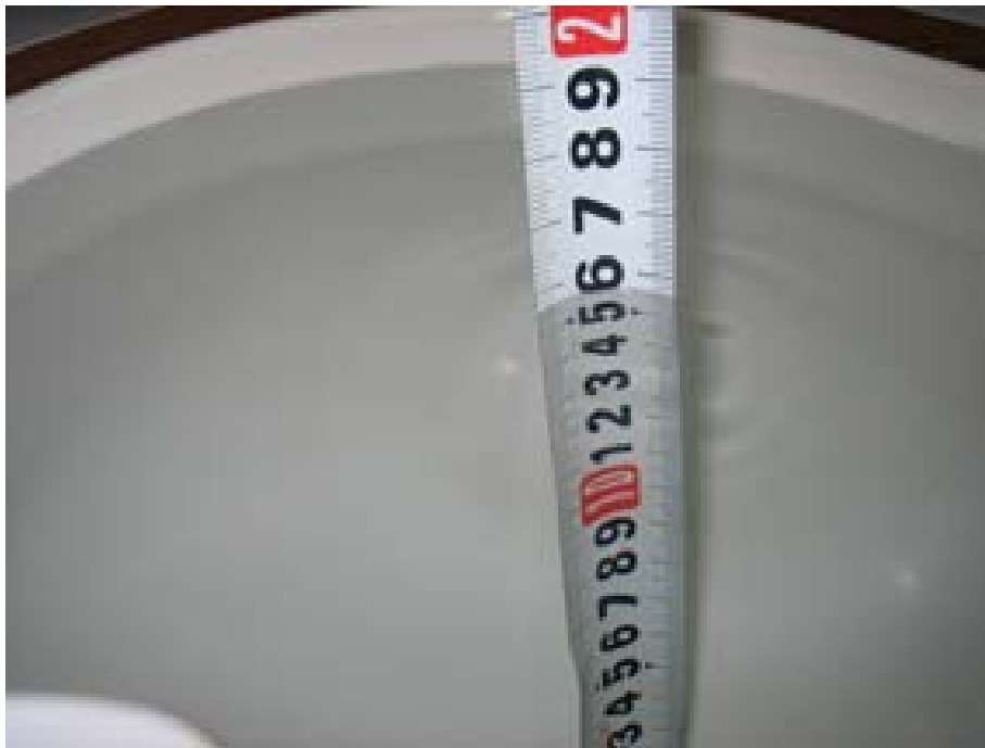
Picture 9 Liquid Depth at Ear Reference Point for 1900MHz Head Liquid
