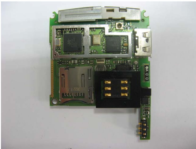
Picture 4: the back view of the PCB with the shielding cover removed
