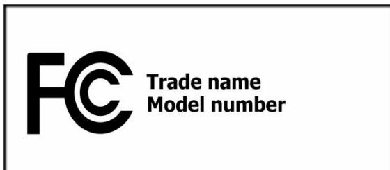
When the device is so small or for such use that it is not practicable to place the statement specified under paragraph 15.19(b)(1) on it, such as for a CPU board or a plug-in circuit board peripheral device, the text associated with the logo may be placed in a prominent location in the instruction manual or pamphlet supplied to the user. However, the unique identification (trade name and model number) and the logo must be displayed on the device.
